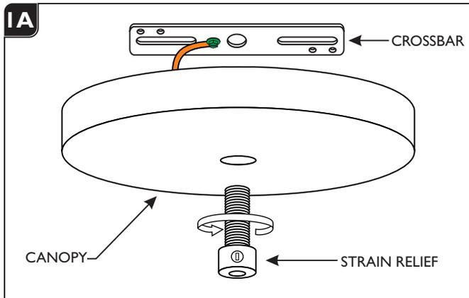
**1** Remove the crossbar from the canopy by completely unscrewing the strain relief.
