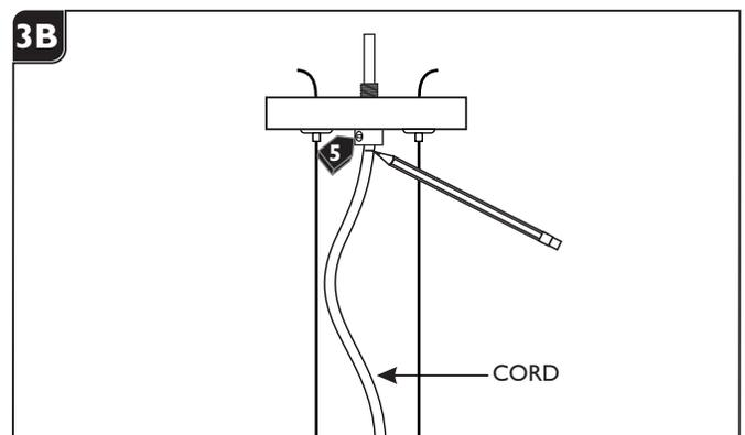
**NOTE:** The power cord does not support the fixture. For a casual "lazy cord" look, cut the power cord several inches longer than the drop height of the fixture.
