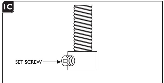
**3** Loosen (**Do Not Remove**) the set screw on the strain relief.
