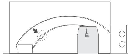
10. Insert can in the housing and fix it with the two adjustment screws.
