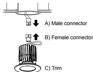
Push connected wires in the pot then push the trim in the can.
