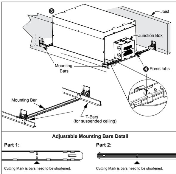
5. Bring the electrical wiring to the housing junction box as per applicable local electrical codes.
